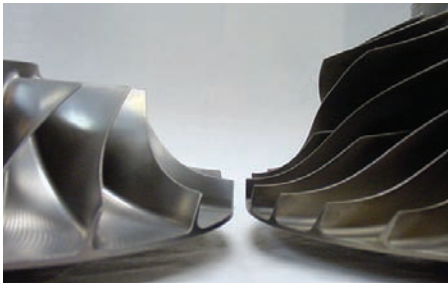
Larger compressor improves pneumatic performance
